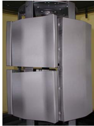
Fig.1 CMSII industrial coating unit and a load of CFC divertor tiles coated with 20 μm of tungsten
