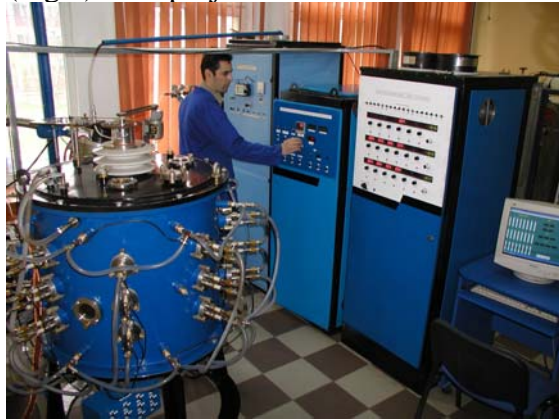
Fig.1 CMSII industrial coating unit and a load of CFC divertor tiles coated with 20 μm of tungsten
